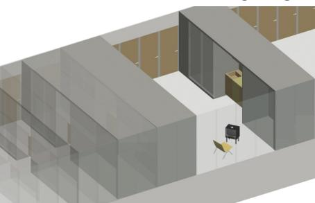
The RTL flat is defined as the void between 2 deep partition walls, which contain all the tenant's items, devices and equipment. The walls can be shifted sideways. So, instead of many smaller spaces with specific functions, this dwelling is a singular, dynamic space with a function momentarily determined by the equipment selected from the walls.
